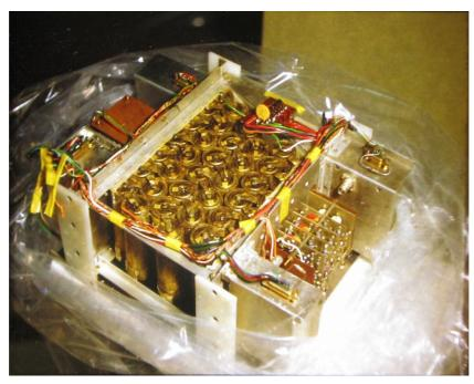
You can see the large battery pack in the centre, dictating the moments of inertia. The magnet was along the maximum dimension below the batteries and is not visible in this picture. Other metals were stainless steel and aluminium, and so did not interfere with the magnet's effect. Here's a diagram showing the placement of components:
